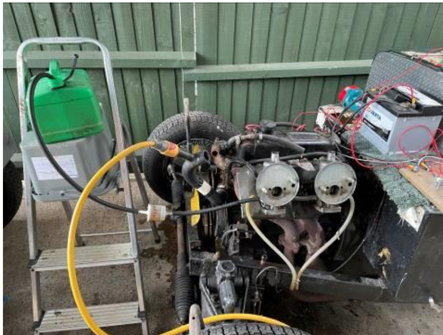
The Jury rigged engine start.
