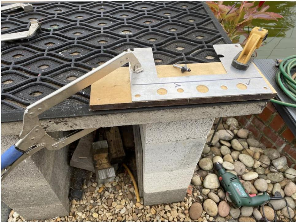
**Set up for routing the edges.**
