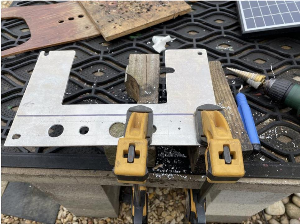
**Cutting the holes with a step drill.**
