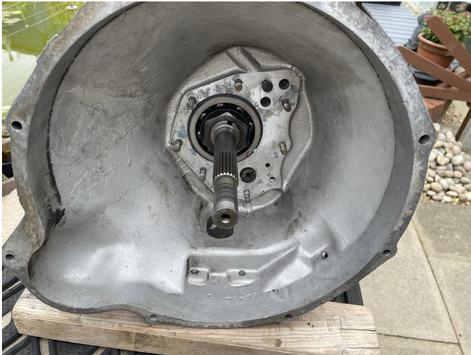
Oil seal cover removed.
