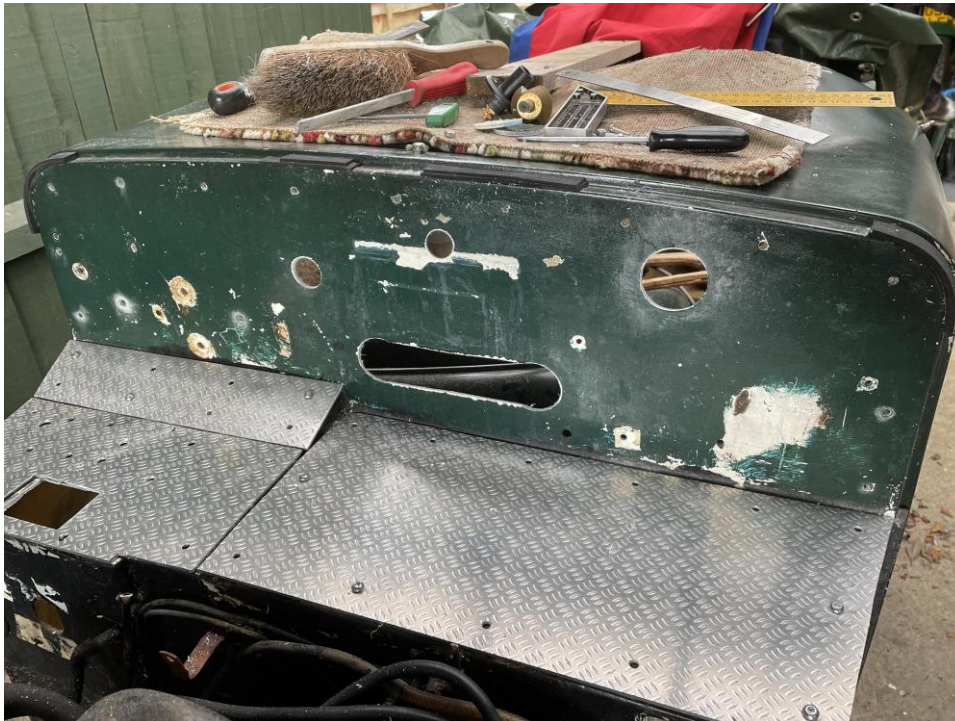
Additional holes made in the fibreglass bulkhead.
