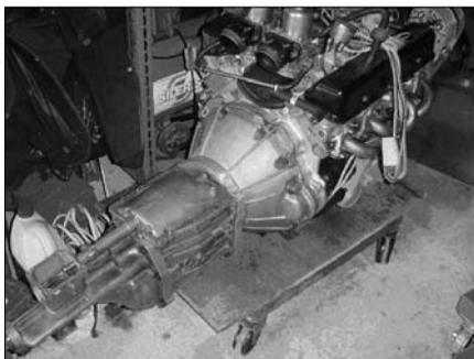
Figure 9 - Gearbox fitted to engine
