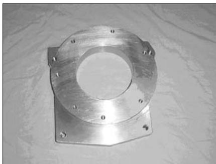
Figure 7 - Completed adapter plate
